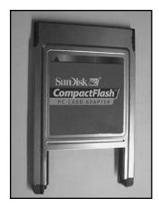
The Back Up Adapter allows the removable memory card to be installed in the PCMCIA card slot of a Laptop PC. When this is done a back up may be made of the customer database. This item is available from www.sandisk.com or Insight Direct.
