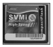
The Data Storage device consists of Compact Flash (CF). The current size of this CF is 256 MB. This allows for the Operating System, Application Software, and all the Prompts, Greetings, and Message Storage. The CF for the SVMi-4E is available only from SAMSUNG.
